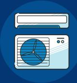
Air source heat pumps extract heat from outside air that is then used for heating indoor spaces during the colder months. They can also extract heat from indoors and expel it outside to cool indoor spaces during the warmer months. Air source heat pumps like a ductless mini-split can be used to heat or cool single rooms (partial load) and whole homes (full load).
