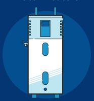
Heat pump water heaters extract heat from the air surrounding the unit to heat water. They can replace electric or fossil fuel-powered water heaters that require much more energy to run efficiently—leading to big savings.
